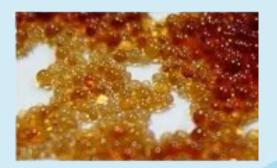
Strong acid cation (SAC) exchange resins are ion exchange resins that are commonly used in water treatment systems. They are used to remove hardness ions like calcium (Ca2+) and magnesium (Mg+) from water. They are composed of a polymer matrix to which anionic functional groups are bound, such as sulphonate (SO3-). SAC resins are regenerated with either a sodium salt solution (Na2+) for softening applications.
