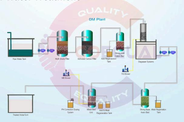
DM Plant is an Ion exchange technology used to remove salts (cations and anions) from water.
